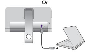
(SW271) The USB-C<sup>™</sup> port on the monitor transfers data only and does not support power delivery to the laptop. Additional power supply to the connected laptop is required.
