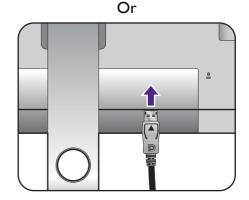
After the monitor and the computer are powered on, if the image is not displayed, disconnect the DP cable. Connect the monitor to any video source other than DP first. Go to System and DisplayPort on the OSD menu of the monitor and change the setting from 1.4 to 1.1. Once the setting is done, unplug the current video cable and re-connect the DP cable. To go to the OSD menu, see Basic menu operation on page 43.
