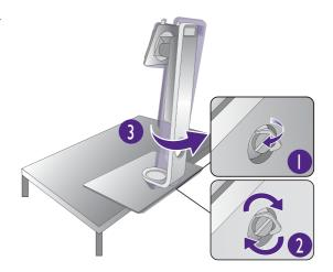
Orient and align the stand arm with the monitor (1), push them together until they click and lock into place (2).
